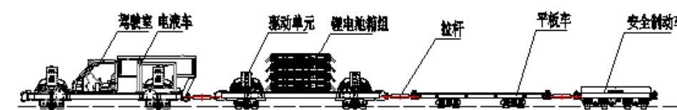
4-wheel drive locomotive layout diagram 1
