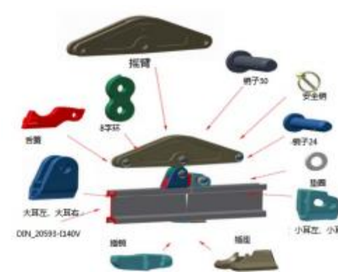
Standard heavy-duty straight rail assembly drawing (Type A)
